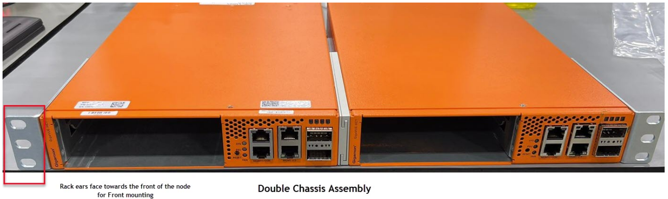
Figure 6 Rack Ears for Front Mount (Reverse Rack Ears for Center Mount)
